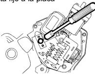
(C) The Delay Assembly consists of two sections nested together and connected by an Orange wire.
