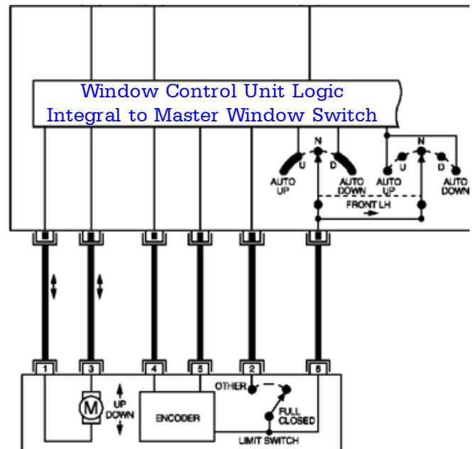
Reset & Limit Switches, Plus Additional Electronics in Motor/Regulator
